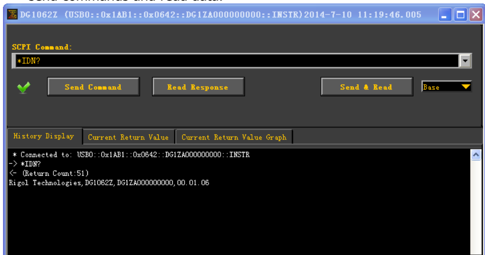
Figure 12 Send and Read Commands via USB
